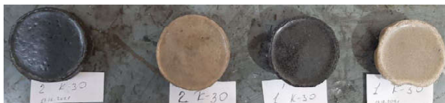
Fig.2. HDPE samples: 1-with graphite filler, 2-with kaolin filler, 3-graphite+kaolin+modified fibrous filler, 4-fibrous filler
